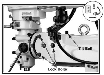
Figure 25. Head tilting controls.
